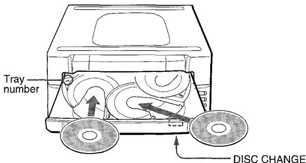
**To load three to five discs,** press DISC CHANGE to rotate the trays after placing two discs. Place the next disc on empty tray. Each time DISC CHANGE is pressed, the trays rotate and one disc can be placed.
